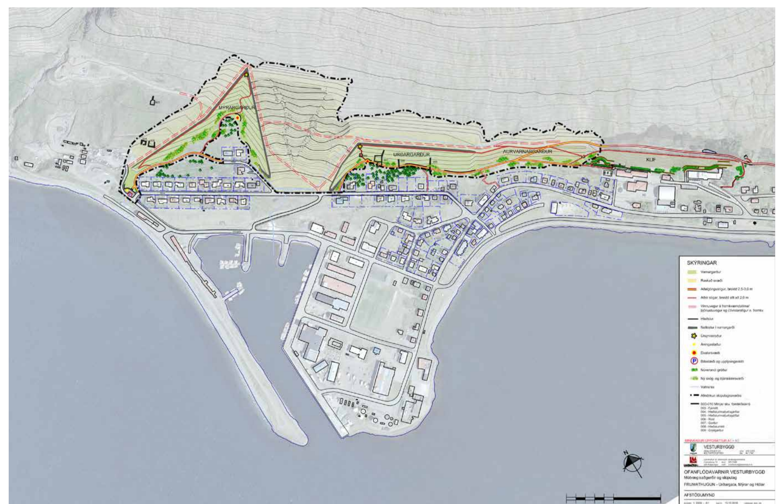
Figure 3. Planned deflecting dams and catching dams in Patreksfjörður, NW-Iceland.
