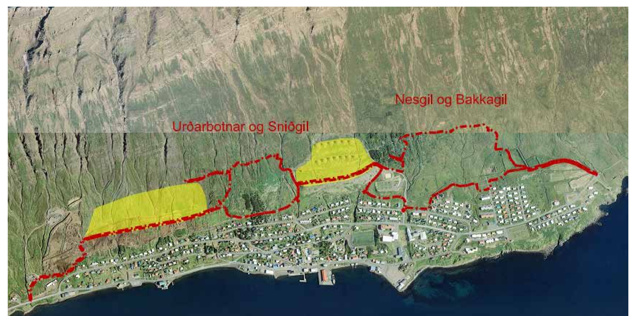
Figure 1. Planned catching dams and braking mounds under Urðarbotnar and Sniðgil and Nes- and Bakkagil in Neskaupstaður, E-Iceland.
