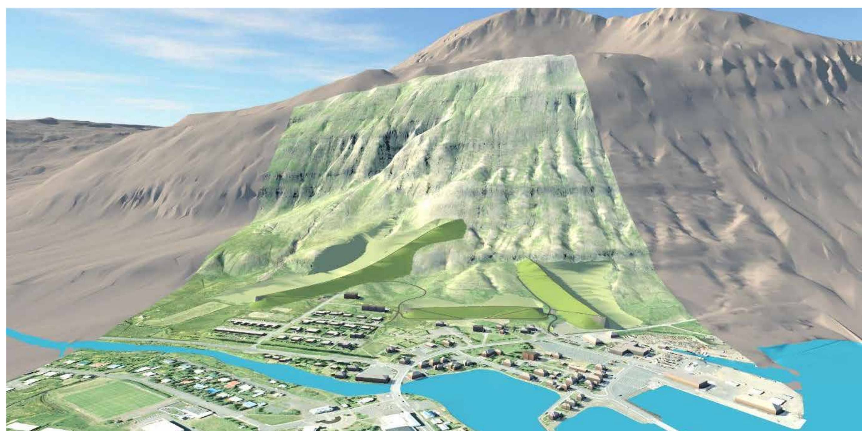
Figure 4. Planned deflecting dams and catching dams in Seyðisfjörður, E-Iceland.
