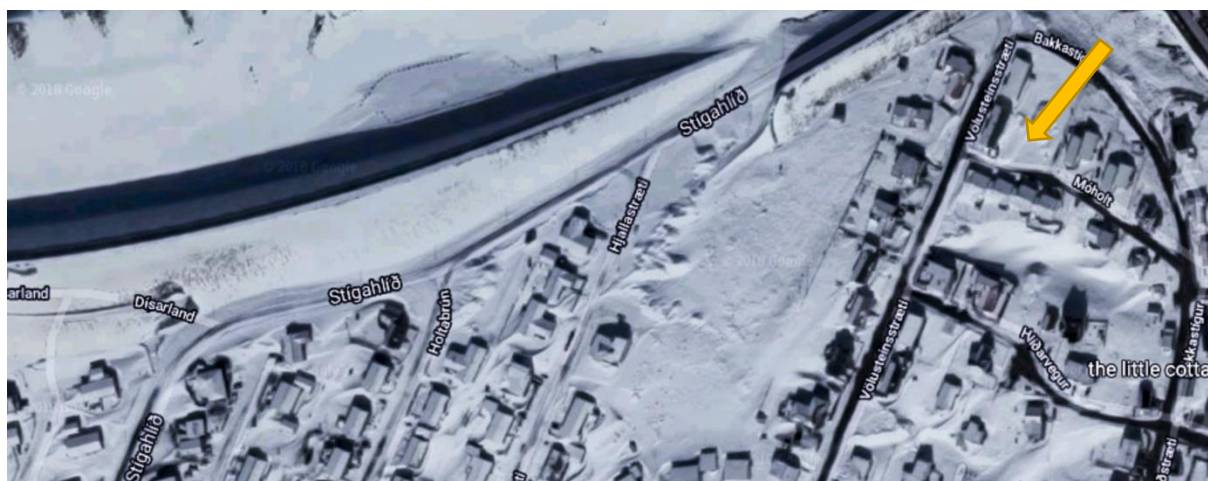
Figure 5 Snow drifts around houses and catching dams in Bolungarvík Iceland after a storm period; wind was blowing from upper right corner to the left, see yellow arrow. Source: Google.com/Maps.
