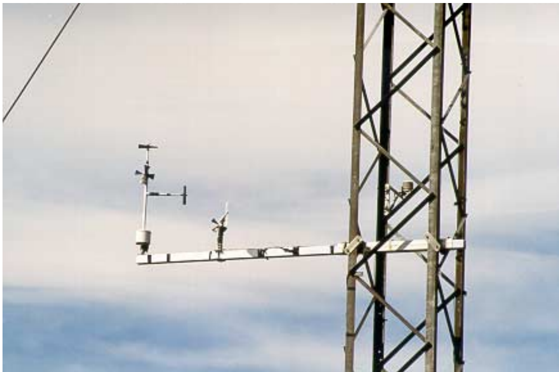
Fig. 2. Anemometers and thermometer at 10.3 - 10.8 m above the ground at Sómastaðagerði. Photo: Flosi Hrafn Sigurðsson, 1999.
