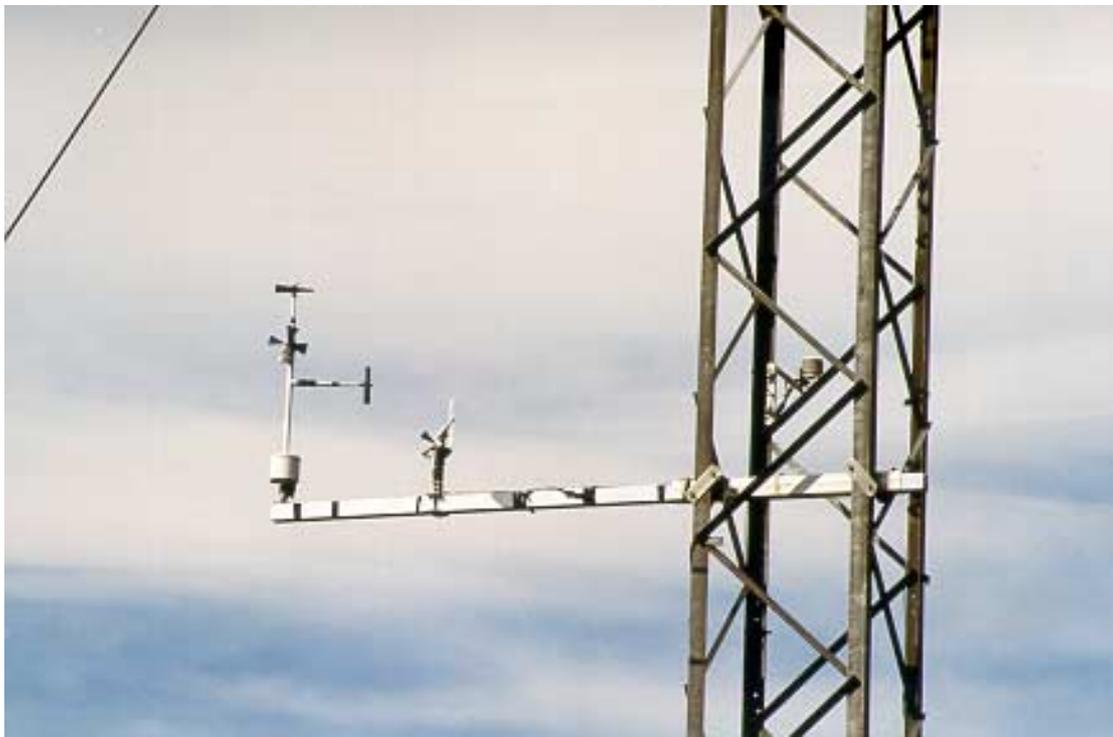
**Fig. 3.** Anemometers and thermometer at 10.3 - 10.8 m above the ground at Sómastaðagerði.
