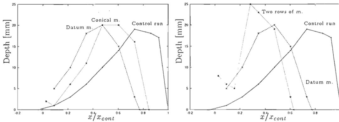
Figure 40: Averaged length profile for conical mounds and two rows of mounds.
