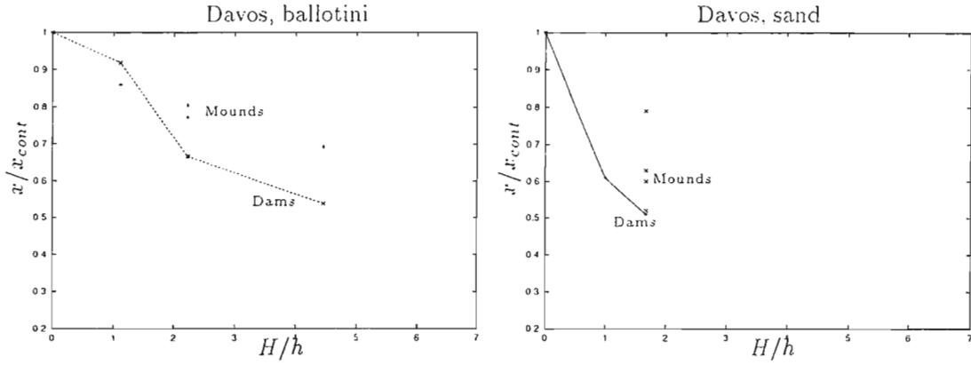
Figure 36: Non-dimensional runout,  $x/x_{cont}$  plotted against non-dimensional heights of the obstacles,  $H/h$ . Datum m. c. stands for datum mound configuration and is defined in Fig. 35.
