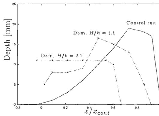
Figure 39: Averaged length profile for the dams.
