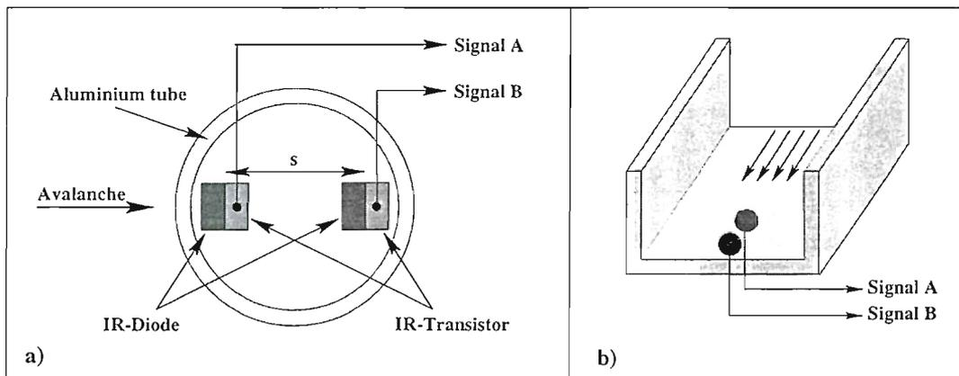
Figure 16: a) Top view of an optical speed sensor. The tube also contains the electronics running the sensors. b) The optical sensors are mounted flush to the sliding surface of the chute.  $s$  is the spacing between the the diode/transistor pairs.
