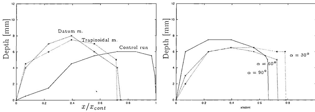
Figure 50: Averaged length profile for trapezoidal mounds and the narrow mounds with different upstream angles,  $\alpha$ .
