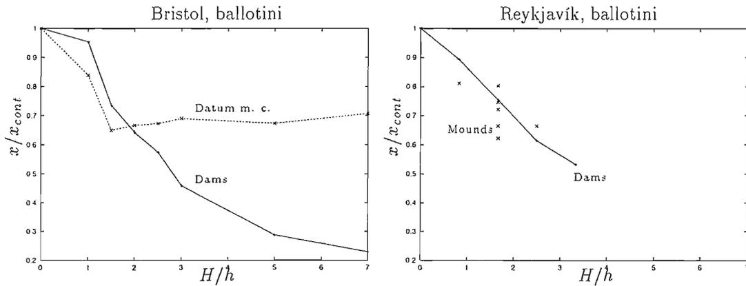
configuration shortens the maximum runout by about 30% for a single row of mounds. The sand experiments also show a similar trend. The most effective single row mound configuration shortens the maximum runout by about 50% and is approximately as effective as a dam of the same height.
