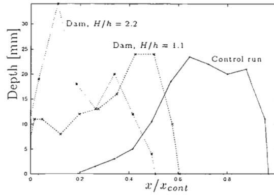
Figure 43: Averaged length profile for the dams.
