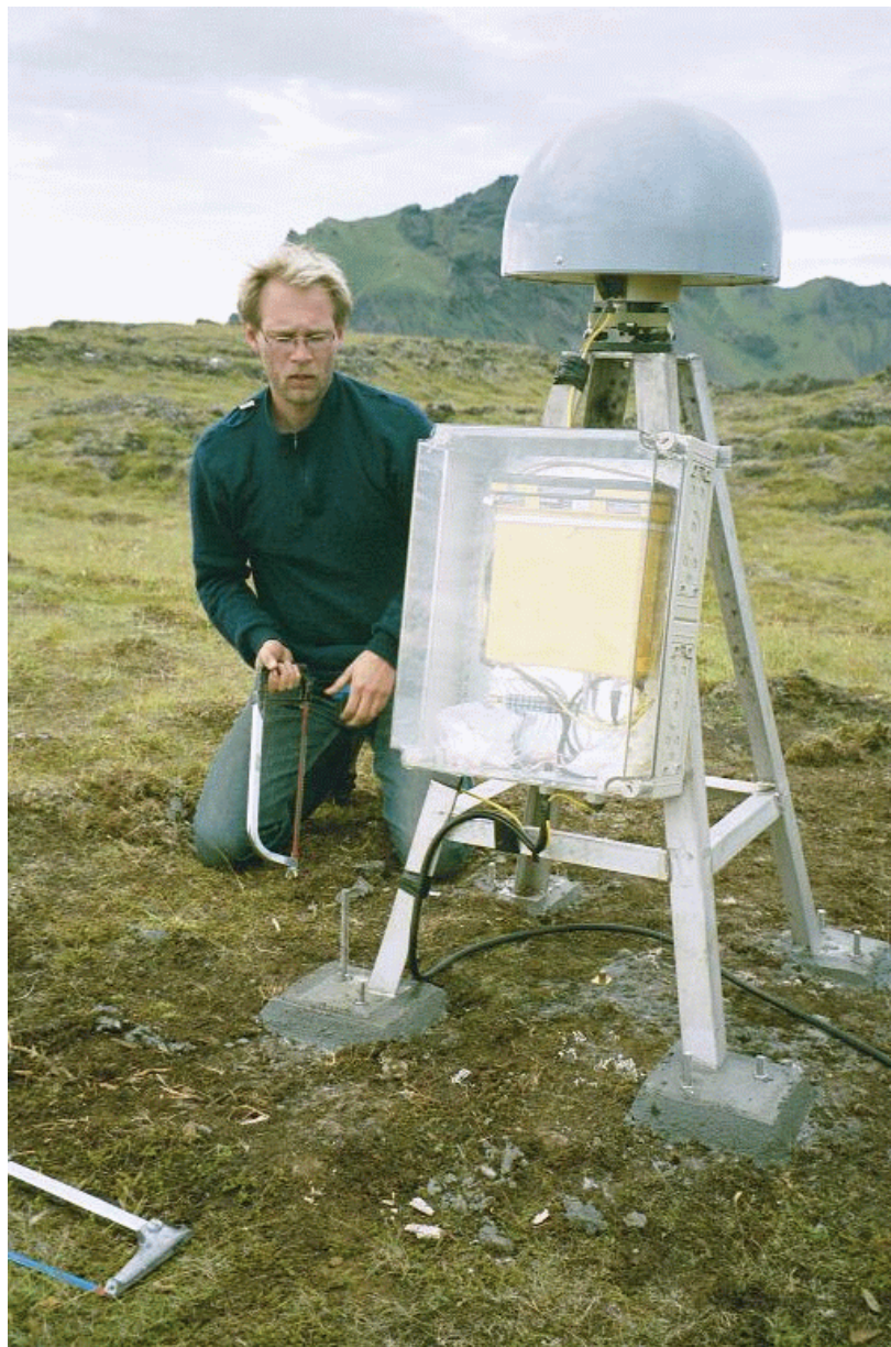
Figure 3. Author finishing the installation at VMEY. If the photo prints out well the brass geodetic benchmark is visible under the center of the quadripod. The antenna is covered with a SCIGN radome (grey plastic) and is mounted on a Leica tribrach. The receiver is mounted in a plastic box screwed to the side of the quadripod. The black cable visible on the ground is the power and data cable coming from a nearby house. The pins seen at the legs of the quadripod are drilled 11 to 22 cm into the bedrock. Concrete visible at the base of the legs is merely for cosmetics. The legs have uneven height from the ground because the top plate of the quadripod is levelled. (Photo: Jósef Hólmjárn).
