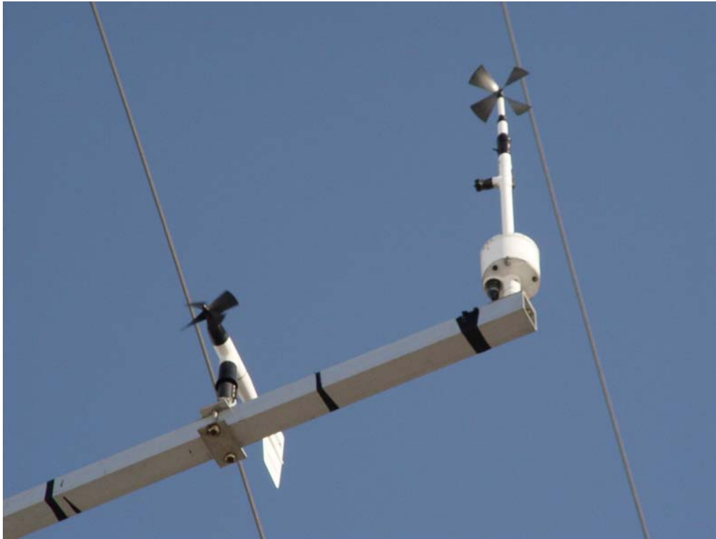
Fig. 4. Young anemometer at 10.3 m height at Sómastaðagerði (left) and Gill vertical component at 10.8 m height (right). Photo: Sigvaldi Árnason, 2003.
