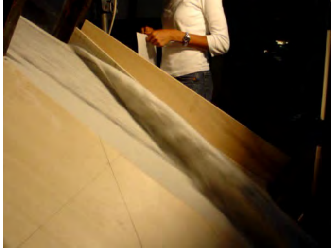
Figure 9: A granular avalanche with Fr \approx 13.5 hitting a deflecting dam with \phi = 20^\circ in a laboratory chute at the Hydraulics and Environmental Engineering Dept. of the University of Pavia.
