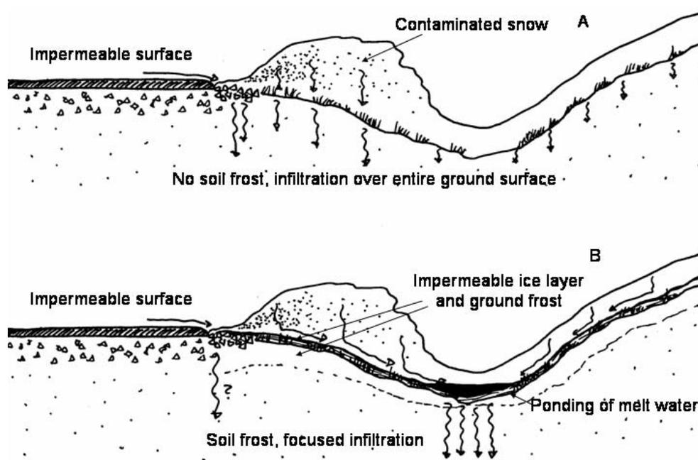
Figure 1. Meltwater flow paths in vicinity of roads or runways A) without soil frost and B) with soil frost.
