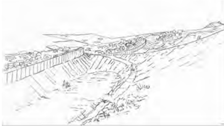
Figure 5 A hand-drawn sketch by Reynir Vilhjálmsson of a catching dam in Siglufjörður, N-Iceland.
