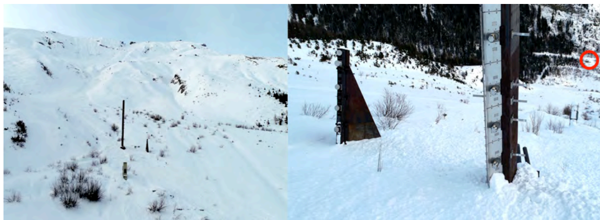
Figure 1. The Vallée de la Sionne test site. The left panel shows the obstacle zone and the release area. The right panel shows the measurement setup at the 20 m high pylon and at the 5 m high wedge. The red circle indicates the position of the shelter with the GEODAR radar (Pictures P. Huguenin).
