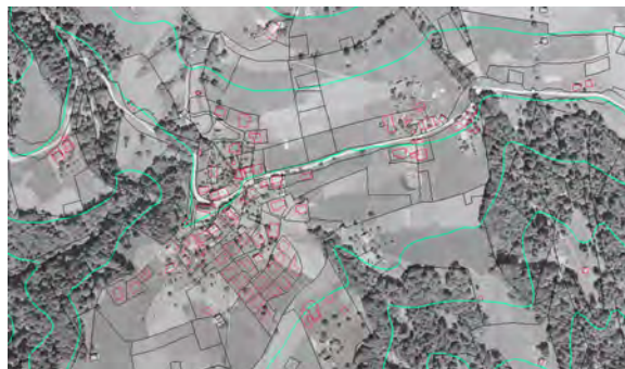
Figure 9: Settlement concentration at the avalanche technically safest place in Blons. The red framed areas are the residential buildings as of 2016. The aerial photo is from the 1950s. The turquoise lines represent contour lines. [VOGIS]
