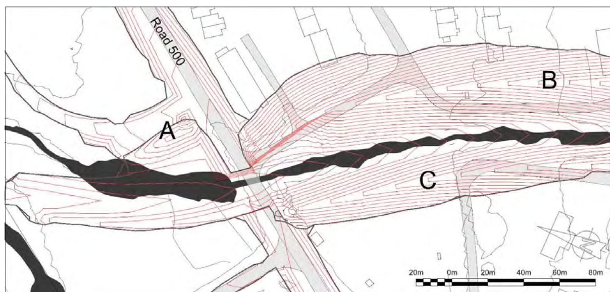
Figure 2 The figure shows Vannledningselva (dark shapes), Road 500 and the planned deflecting dams on both sides of Road 500 (red contours). Letters A-C depict top of dams. The distance between contour lines at the dam is 1 m. This digital elevation model of the deflecting dams was used in the wind simulation in early stage, but the final design will be somewhat different at Road 500, but it is expected that the main principles will be the same. The model shows the cut through road 500 for the river.
