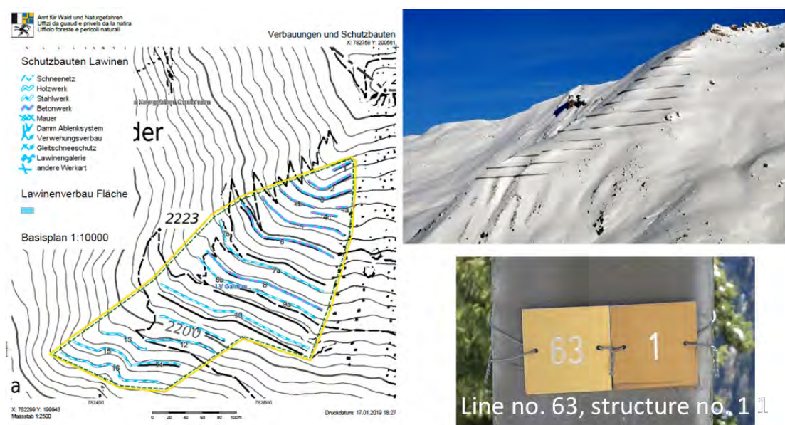
Figure 7 Protective structure register Canton Graubünden with extract of the map server, overview photo and structure numbering
