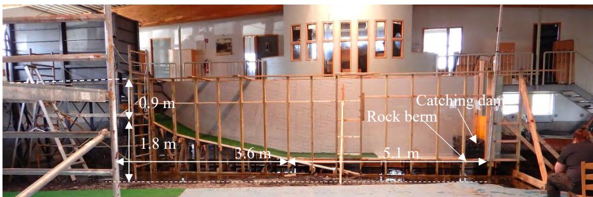
Figure 3 Setup C.6. The experimental chute is 9 m long and 1.2 m wide with a 6 m 3 tank.
