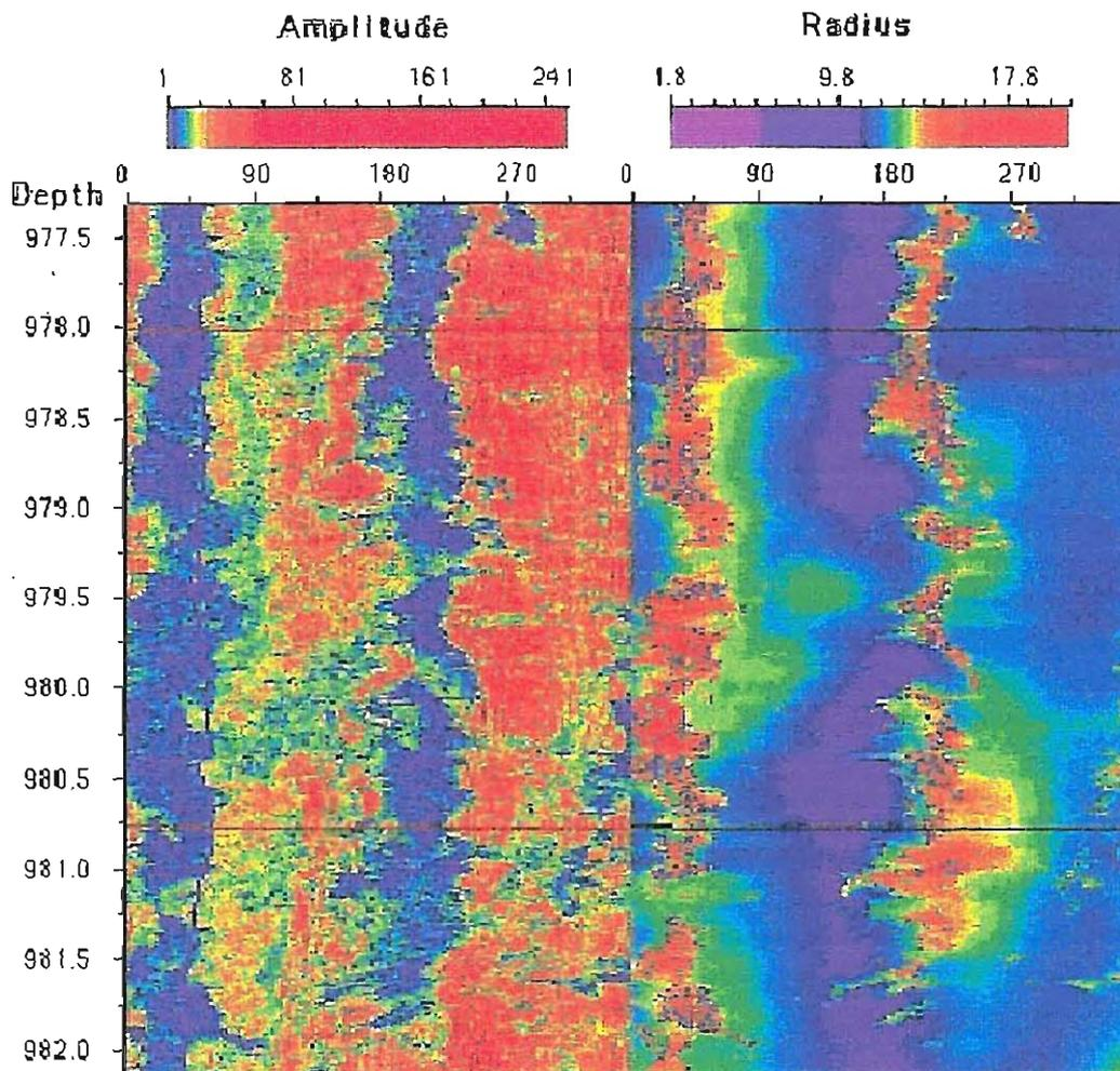
Figure 12: *Televviewer logs run in borehole LL-03 in a depth interval containing breakouts.*
