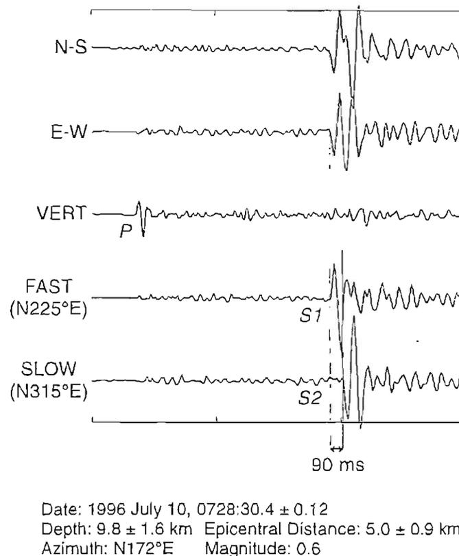
Figure 10: Three-component seismograms of an earthquake (at 07:28:30.4, July 10, 1996) at SAU with time marks at every second. Upper traces are N-S, E-W, and vertical components. The lower traces are horizontal components rotated to the faster (N225°E) and slower (N315°E) shear-wave polarizations showing time-delays between split shear-waves.
