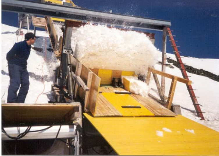
Figure 5: A photograph of the snow hitting a 60 cm high catching dam in the 34 m long chute at Weissfluhjoch. A part of the dam broke during this experiment as seen on the photograph.
