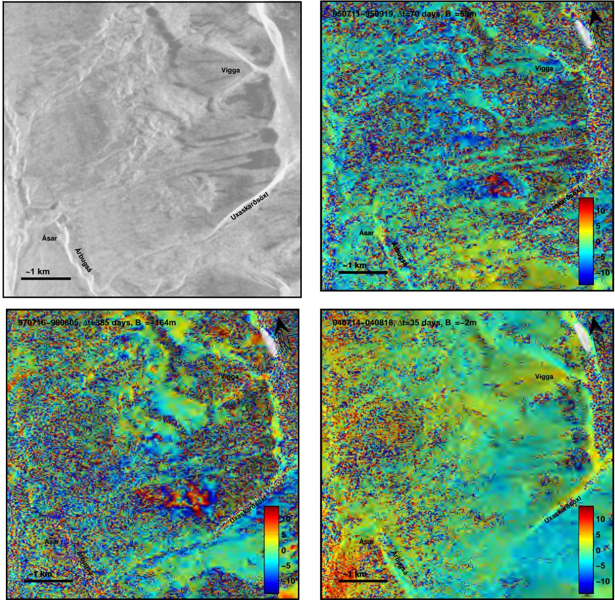
**Figure 16.** A radar amplitude image (top left) and three interferograms of Flateyjardalsheiði. The 70-day interferogram from 1995 (top right) shows clear signs of displacements near Úraskarðsöxl, while the 35-day interferogram from 2004 (bottom right) exhibits no measurable deformation. The one-year interferogram from 1997-1998 (bottom left) is noisier due to the longer time-span but clearly shows deformation below Úraskarðsöxl ©ESA.
