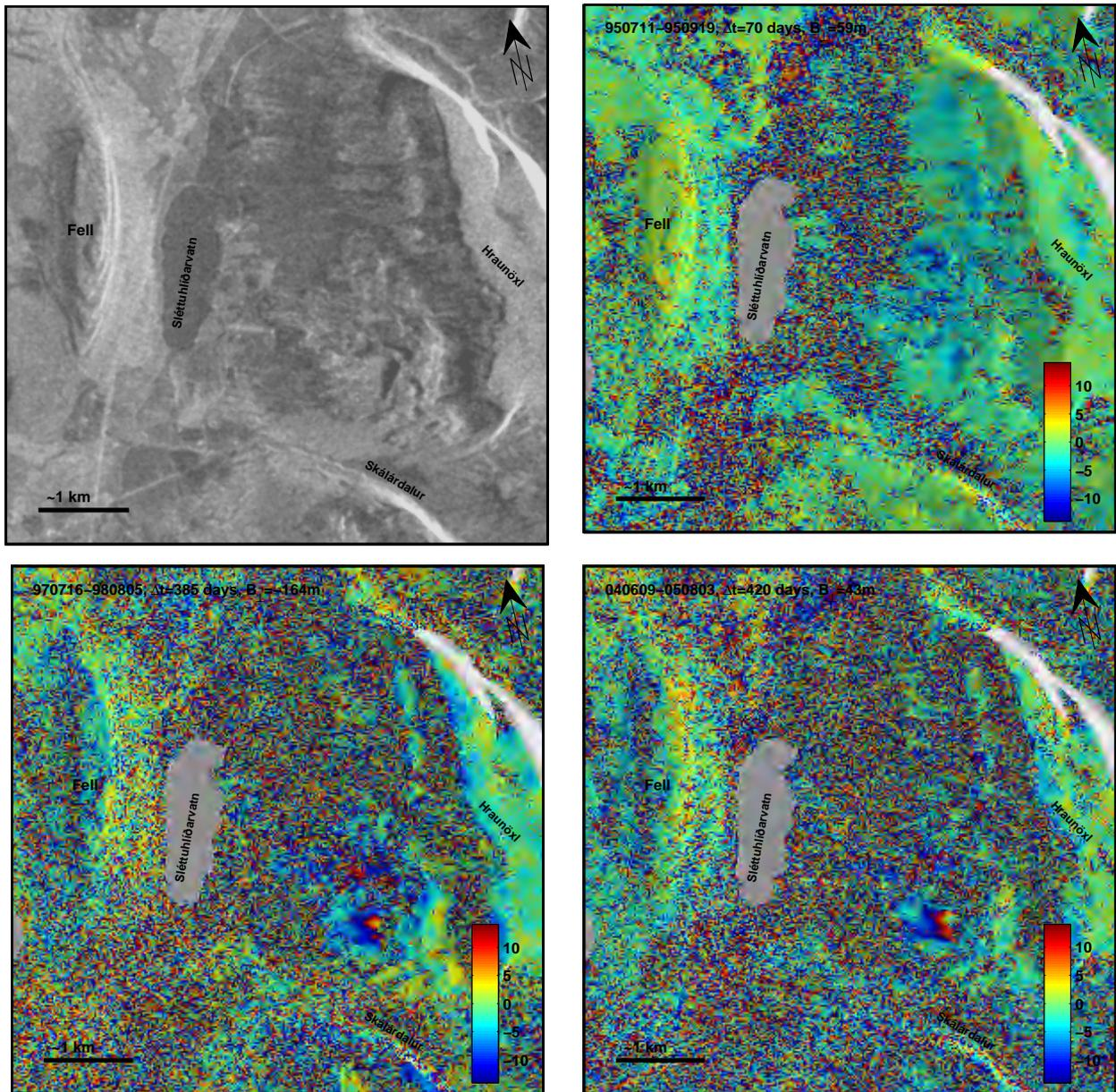
**Figure 30.** SAR amplitude image and interferograms of Sléttuhlíð in radar coordinates. The 70-day interferogram (July-Sept. 1995, top right) exhibits little or no deformation, while the one year interferograms (bottom) from 1997-1998 and 2004-05 show up to 3 cm of displacements on part of the deposits. ©ESA.
