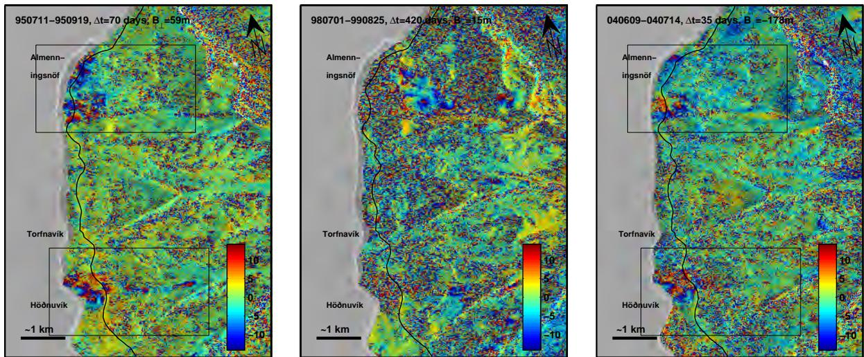
**Figure 13.** Three interferograms of Almenningsnöf spanning two months in 1995 (left), one year from 1998 to 1999 (middle) and one month in 2004 (right). The Siglufjörður road is marked as a black line. ©ESA.
