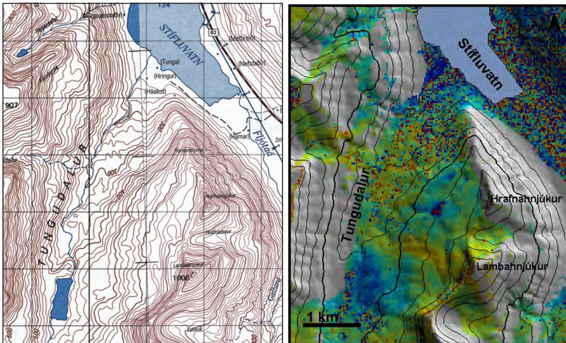
**Figure 27.** Map and a geocoded interferogram (July-August, 2004) of Tungudalur near Stífluvatn showing deformation below Hrafnahnjúkur at 600 m.a.s.l. The interferogram has 100 m contour lines with the 500 m line displayed thick. ©NLSI and ESA.
