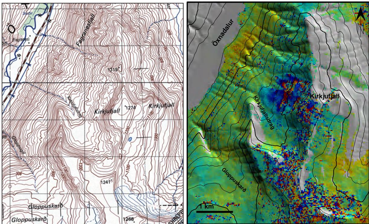
**Figure 22.** Map and a geocoded interferogram (July-August, 2004) of Kirkjufjall in Öxnadalur showing deformation near Kirkjufjallsdrög with 2-3 cm maximum LOS displacement. Both 100 m and 500 m (thick) elevation contour lines are shown. ©NLSI and ESA.
