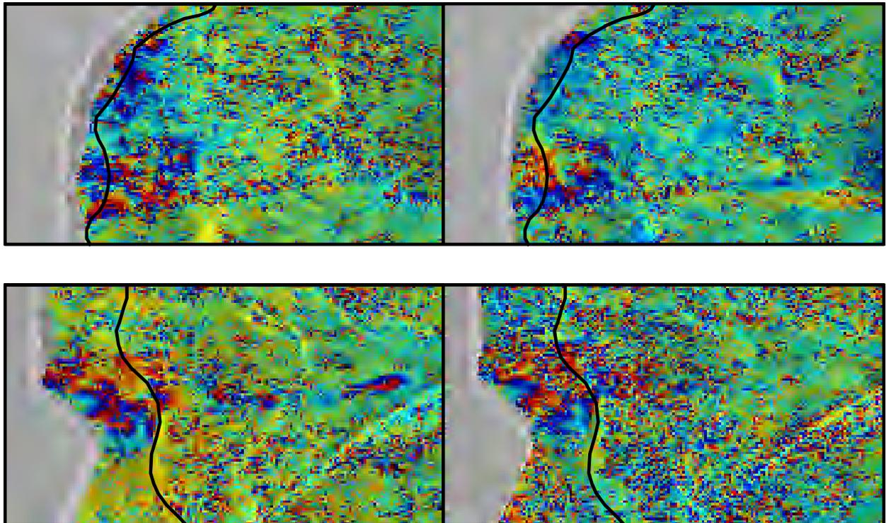
**Figure 14.** Close-ups of the interferograms shown in Figure 13 showing Almenningsnöf (top panels) and the Höðnavík site (lower panels). The interferograms span July-September 1995 (left) and June-July 2004 (right). ©ESA.
