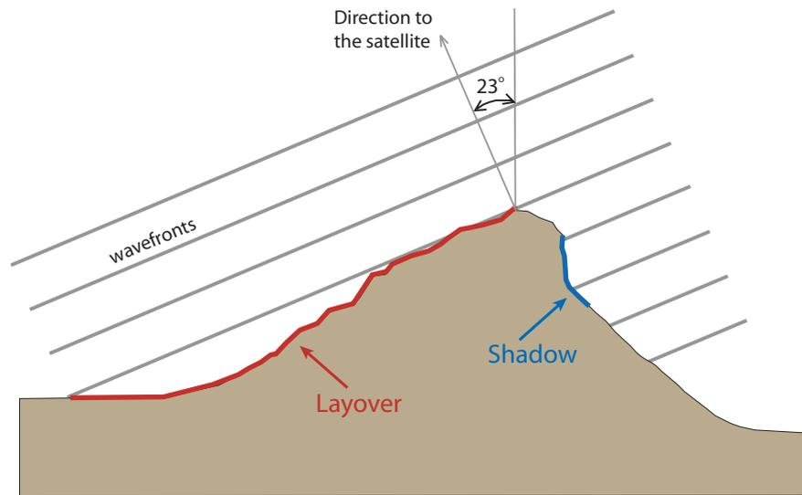
**Figure 2.** Schematic figure showing shadowing and layovers in radar imaging. The gray straight lines indicate incoming wavefronts from a radar satellite looking down from the left. When slopes facing the satellite are steeper than  $23^\circ$  reflected signals from the top of the mountain return before reflections from further down the slope, resulting in a "layover". Slopes facing away from the radar are better imaged, although shadowing can occur on very steep slopes.
