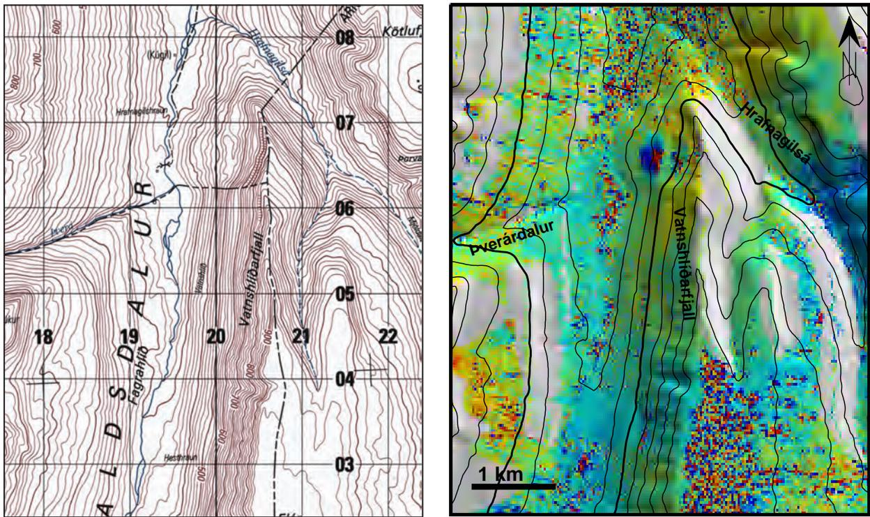
**Figure 24.** Map and a geocoded interferogram of Porvaldsdalur. The 35-day interferogram (July-August, 2004) shows deformation of Hrafnagilshraun. The interferogram has 100 m contour lines with the 500 m line displayed thick. ©NLSI and ESA.
