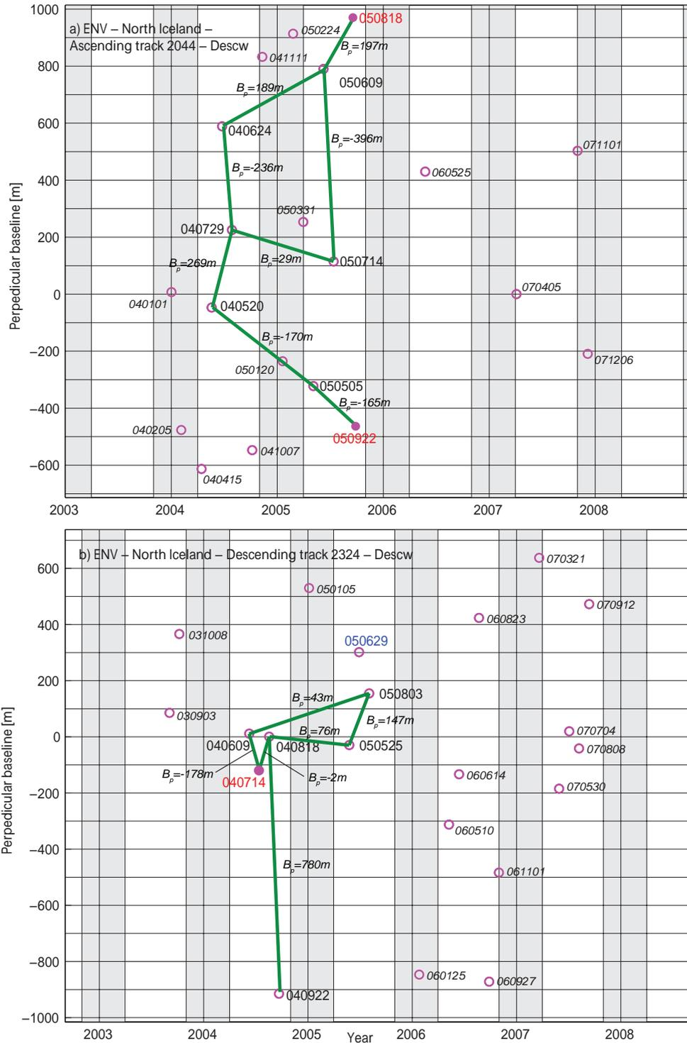
**Figure 7.** A spatio-temporal baseline diagram for Envisat radar data acquired along ascending track 2044 and descending track 2324. Green lines show which interferograms were formed. Scenes in italic script exist, but were not ordered for this project. Scenes labelled in red exist, but are missing in ESA’s Descw catalogue, while the scene in blue (29 June 2005) is listed in the Descw, but does not exist.
