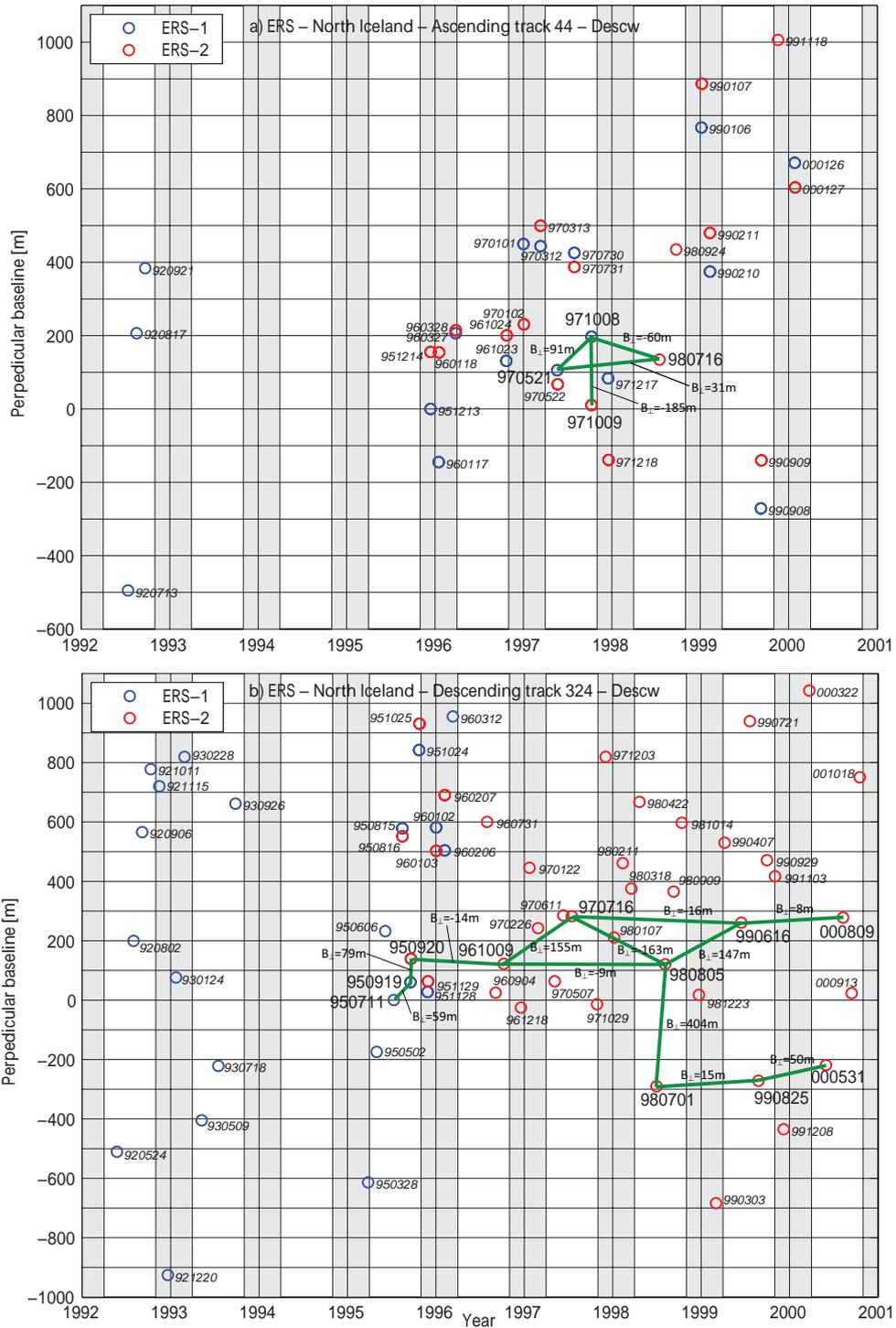
**Figure 6.** Spatio-temporal baseline information for ERS ascending track 44 and descending track 324 for the time period 1992-2001. The information comes from ESA’s Descw database. Scenes labeled in non-italic were ordered for the project and green lines indicate the interferograms formed. Also shown is the perpendicular baseline ( $B_{\perp}$ ) as calculated from the precise Delft orbital information.
