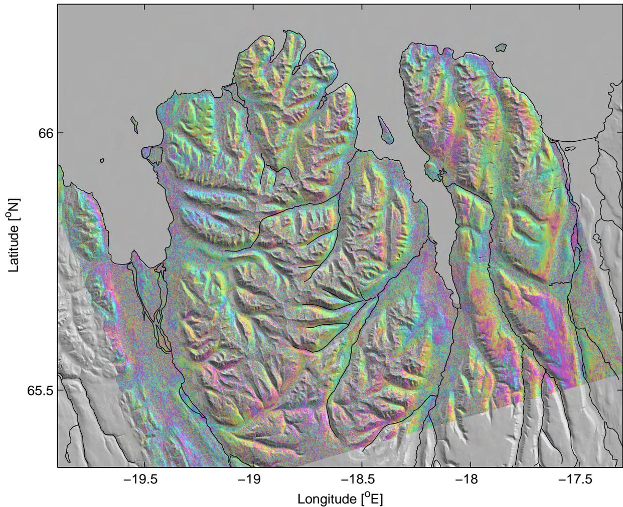
**Figure 8.** *Example of a geocoded ascending Envisat interferogram of North Iceland (9 June - 18 August, 2005). The displayed area is too large to see any details in the data. However, one can see that the interferogram is decorrelated at the lowest elevations, due to vegetation growth and agricultural activities, and at the highest elevations too, presumably due to snow. The main phase variations are from atmospheric effects that correlate with the topography in some places. ©ESA.*
