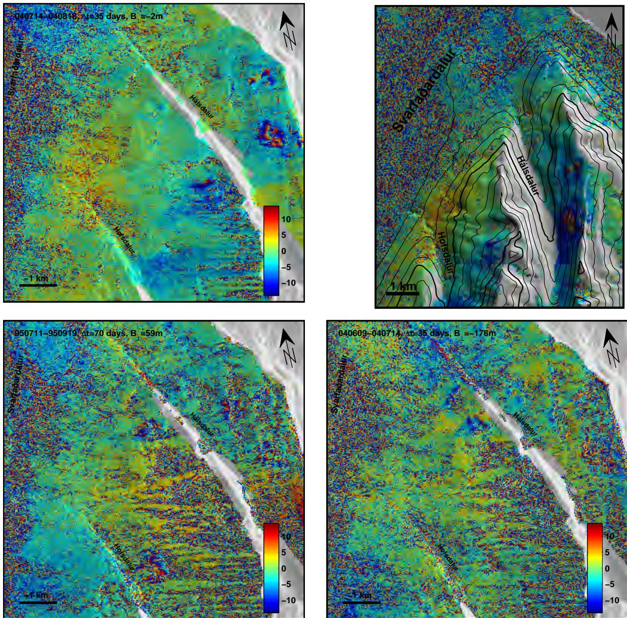
**Figure 26.** Interferograms of Svarfaðardalur. A 35-day interferogram (July-August, 2004), both in geographic and in radar coordinates (top). Two other interferograms spanning 70 days in 1995 (bottom left) and June-July 2004 show the same area in radar coordinates (bottom). ©ESA.
