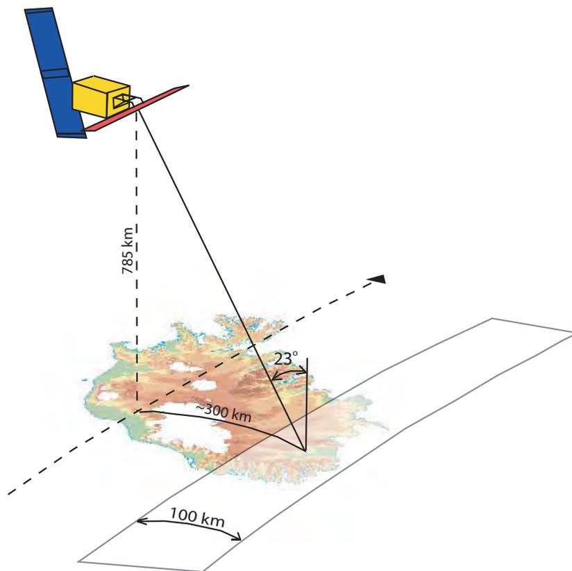
**Figure 1.** Schematic figure of an ERS-2 ascending pass covering East Iceland. The incidence angle is  $23^\circ$  in the middle of the 100 km wide swath the satellite covers in each pass. The viewing direction during ascending passes is about  $N78^\circ E$  for ascending passes and  $N78^\circ W$  for descending passes.
