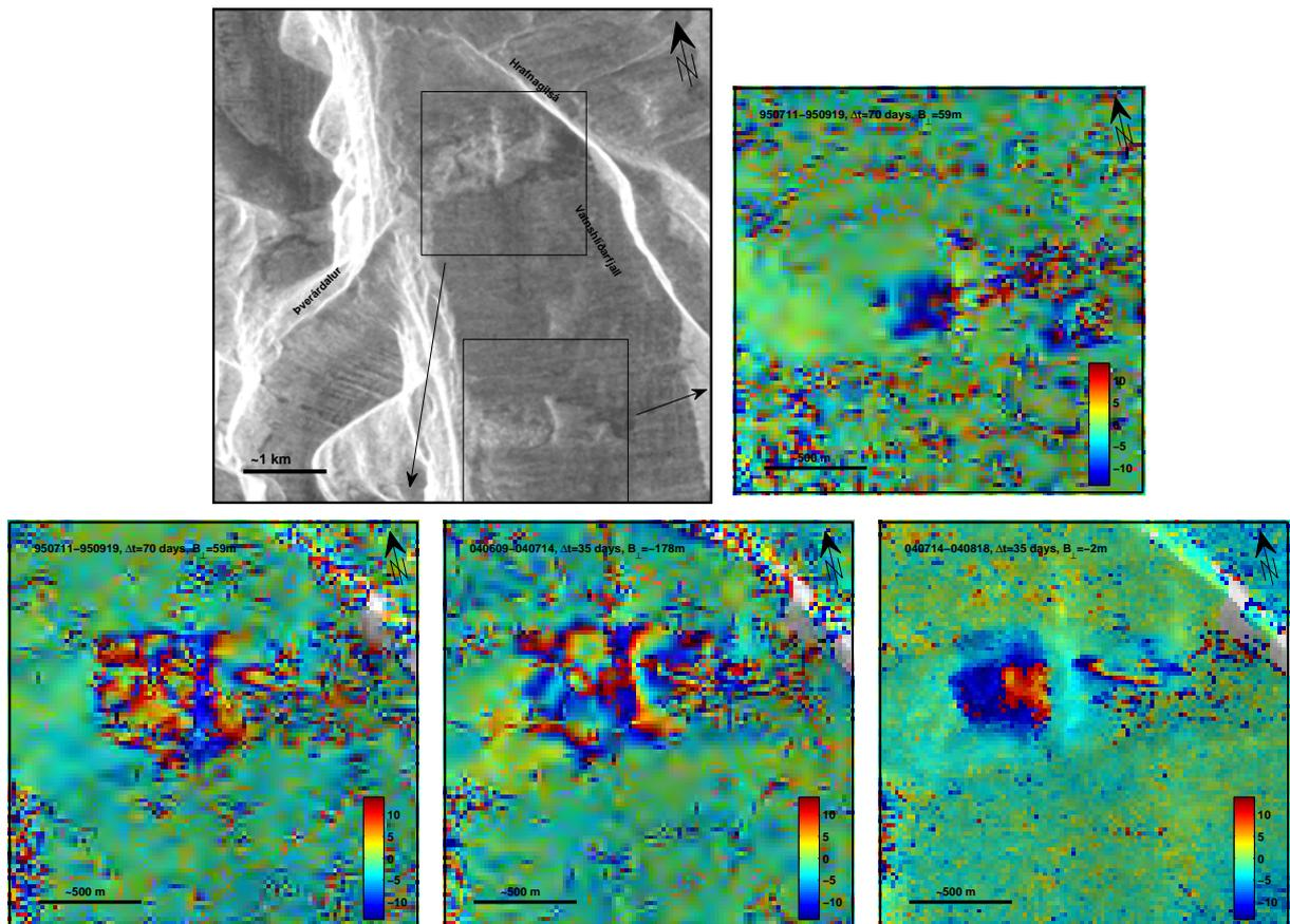
**Figure 25.** Amplitude image and interferograms of Porvaldsdalur. The July-August (2004) interferogram is here shown in radar coordinates (it is in map coordinates in Figure 24) and it shows clear deformation on Hrafnagilshraun (bottom right). Two other interferograms spanning 70 days in 1995 (bottom left) and June-July 2004 (bottom middle) show stronger displacements at the same site as well as hint of displacement further south near Hesthraun (top right). ©ESA.
