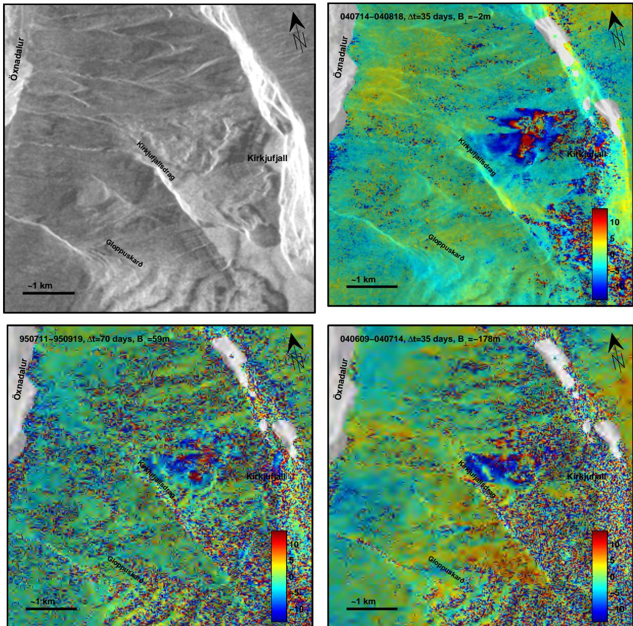
**Figure 23.** Amplitude image and interferograms of Öxnadalur. A 35-day interferogram (July-August, 2004) shows deformation in Kirkjufellsdrög in the radar-geometry (same as in Figure 24). Two other interferograms spanning 70 days in 1995 (bottom left) and June-July 2004 (bottom right) also show displacements at this site. ©ESA.
