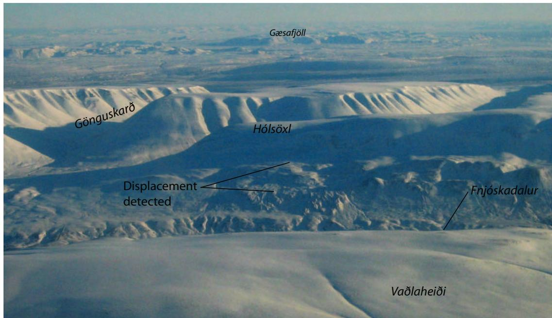
**Figure 17.** Looking east over Vaðlaheiði towards Hólsöxl on the east side of Fnjóskadalur valley. Loose deposits can be seen under Hólsöxl, above and north of the farm Böðvarsnes, and they appeared to be moving in some of the processed interferograms.
