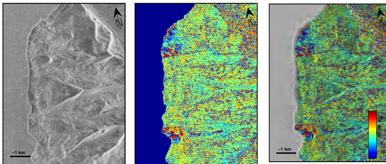
**Figure 10.** *Display example of an interferogram from Almenningur near Siglufjörður. The displayed image includes a SAR amplitude image (left) as a background shading for the interferometric phase observation (middle) and the result is a shaded interferogram (right).* ©ESA.
