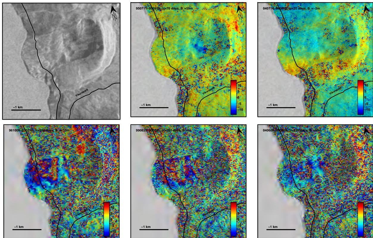
**Figure 21.** SAR amplitude image (top left) and five interferograms of Víkurhólar in Eyjafjörður, two spanning only 70 and 35 days (top middle and right) and three spanning about a year in 1998-99, 1999-2000, and 2004-05 (bottom). ©ESA.
