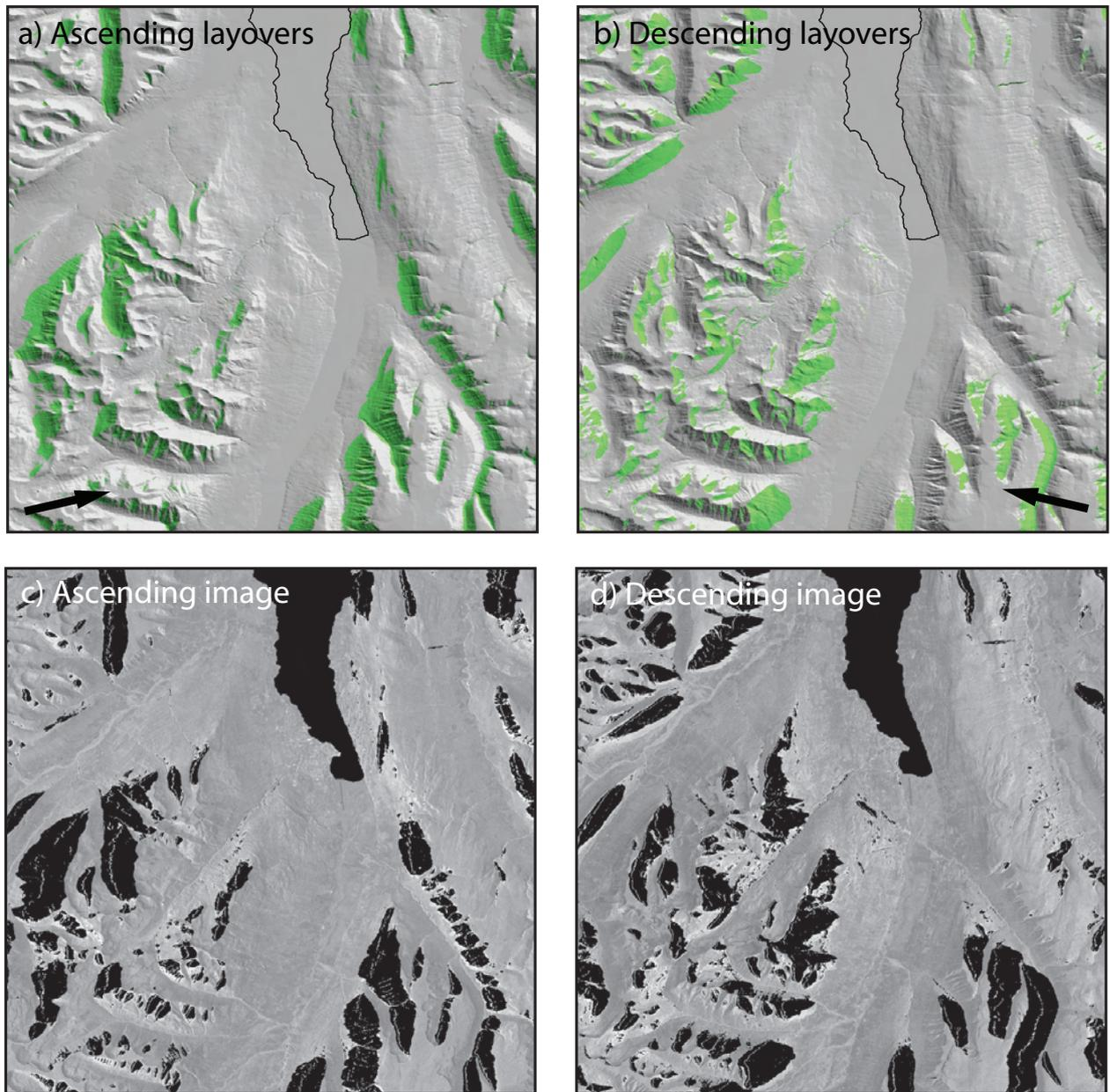
**Figure 4.** Map of ERS-1/2 layovers (shown as green) from the a) ascending and b) descending viewing directions for the same area as in Figure 3. Black arrows indicate the look direction of the satellite. The figures show clearly that many slopes cannot be imaged using only one look direction. c-d) show the corresponding geocoded amplitude images with layover areas masked out.
