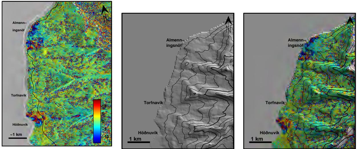
**Figure 11.** *Example of the postprocessing of an interferogram from Almenningur near Siglufjörður: Filtered interferogram (left), shaded relief map (middle), and a geocoded interferogram (right). ©ESA.*
