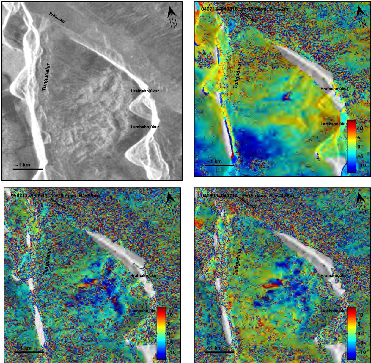
**Figure 28.** SAR amplitude image and interferograms of Tungudalur. The 35-day interferogram (July-August, 2004) is the same as in Figure 27, except it is here in radar coordinates. Two other interferograms spanning 70 days in 1995 (bottom left) and June-July 2004 (bottom right) show stronger displacements at the same site. ©ESA.
