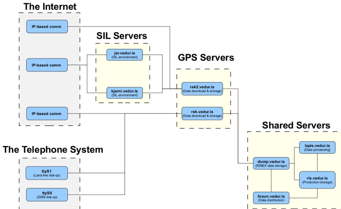
Figure 4. Servers used at IMO to download, process, store and distribute GPS data.
