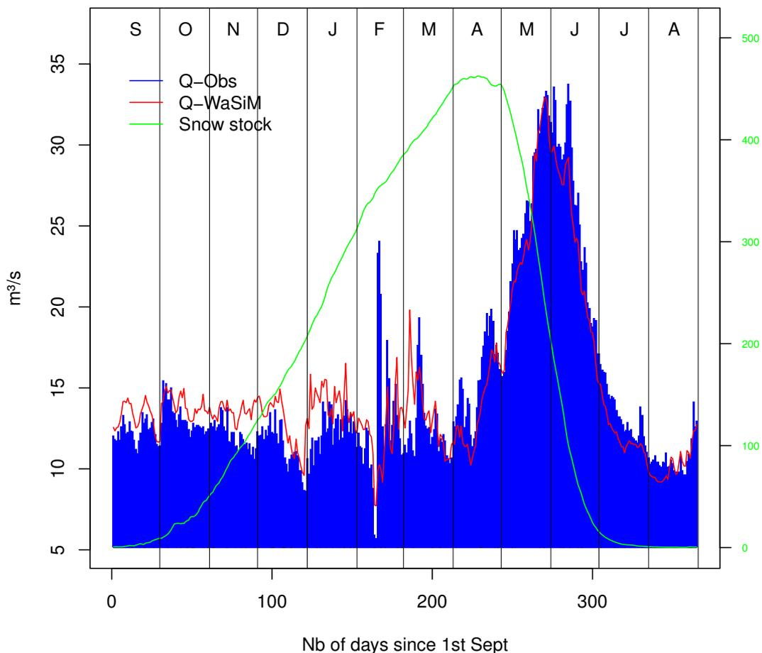
Figure 13. WaSiM-ETH model validation at gauge vhm26. Discharge seasonality: observed (blue), best model simulation (red). Simulated catchment-averaged snowpack (green) (mm SWE).
