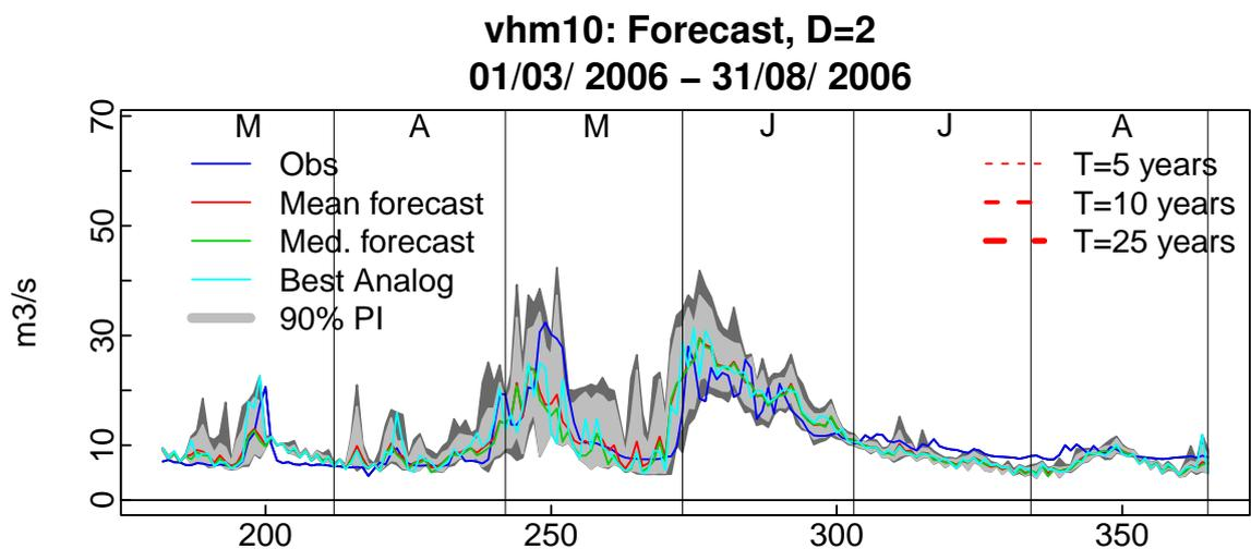
Figure 25. Ensemble daily flow predictions ( $Q_{DMO}$ ) at gauge vhm10 for a lead time of two days ( $D=2$ ), in the hydrological year Sept. 2005–Aug. 2006. The dark grey band corresponds to the dispersion of the ensemble prediction and the light grey band represents the 90% prediction interval.
