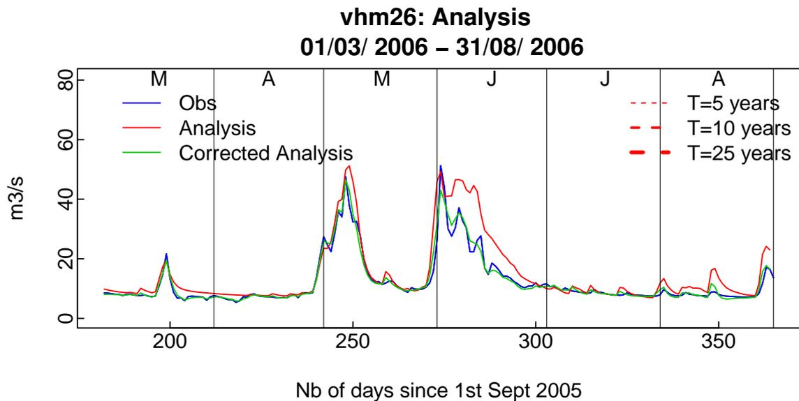
Figure 27. Observed vs. simulated daily discharge in analysis mode ( $Q_{analysis}$ ) at gauge vhm26, in the hydrological year Sept. 2005–Aug. 2006.
