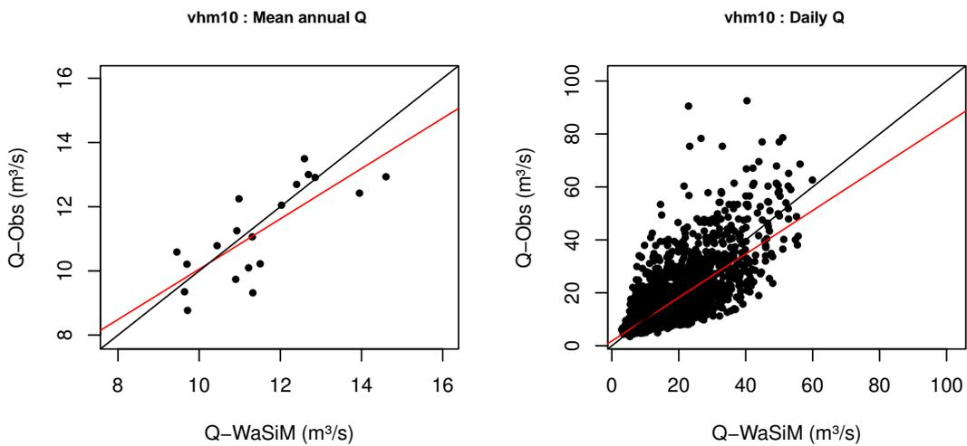
Figure 12. WaSiM-ETH model validation at gauge vhm10. Observed versus simulated discharge. Annual discharge (left), daily discharge (right). The black line corresponds to the 1:1 line and the red line to the regression line.
