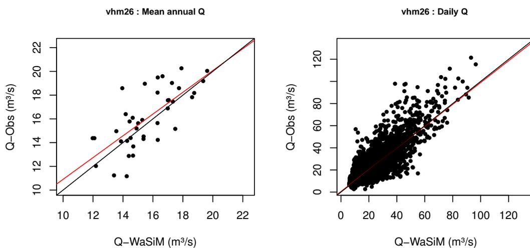
Figure 14. WaSiM-ETH model validation at gauge vhm26. Observed versus simulated discharge. Annual discharge (left), daily discharge (right). The black line corresponds to the 1:1 line and the red line to the regression line.
