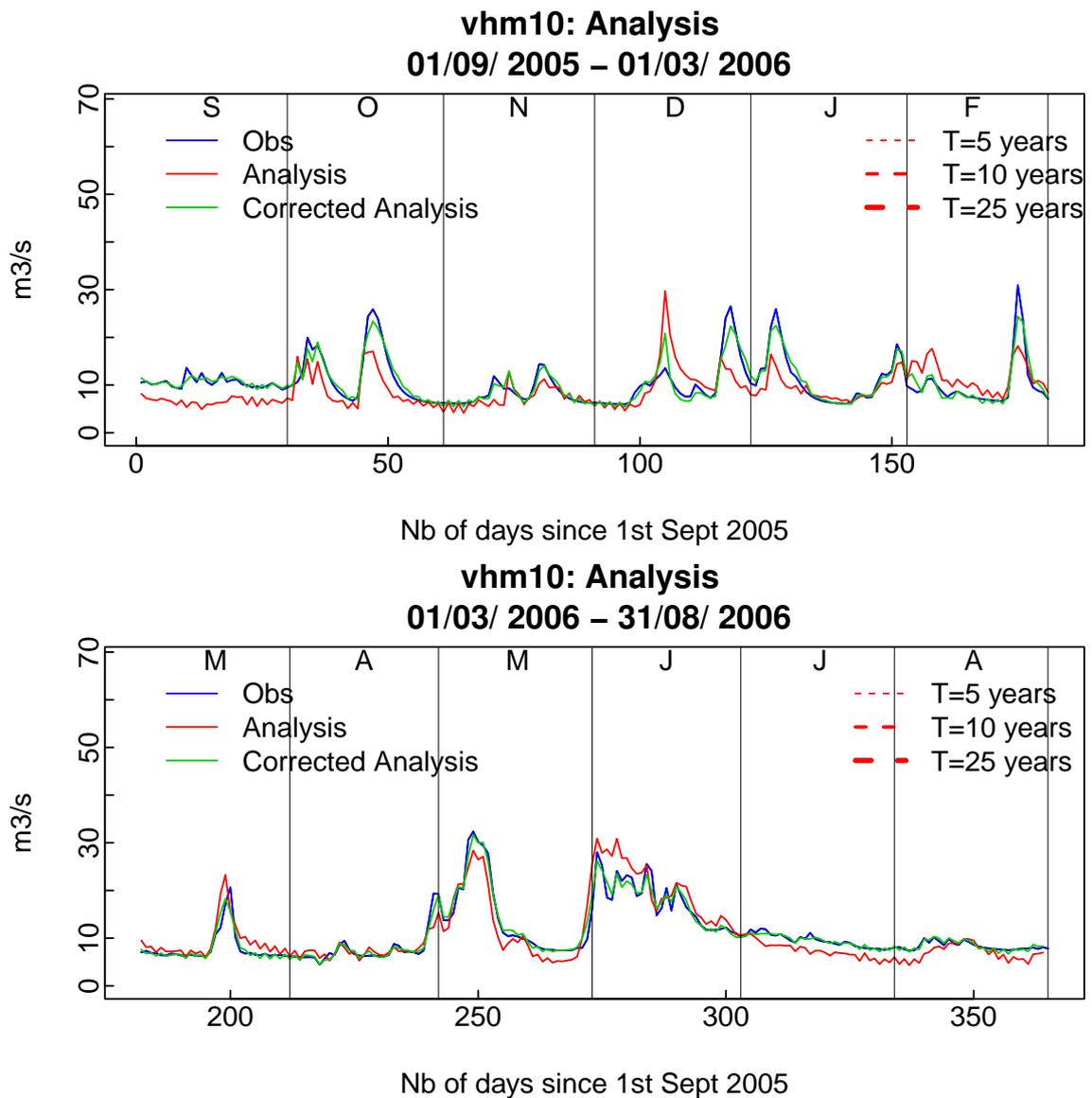
Figure 24. Observed vs. simulated daily discharge in analysis mode ( $Q_{analysis}$ ) at gauge vhm10, in the hydrological year Sept. 2005–Aug. 2006.
