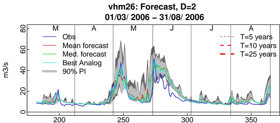
Figure 28. Ensemble daily flow predictions ( $Q_{DMO}$ ) at gauge vhm26 for a lead time of two days ( $D=2$ ), in the hydrological year Sept. 2005–Aug. 2006. The dark grey band corresponds to the dispersion of the ensemble prediction and the light grey band represents the 90% prediction interval.
