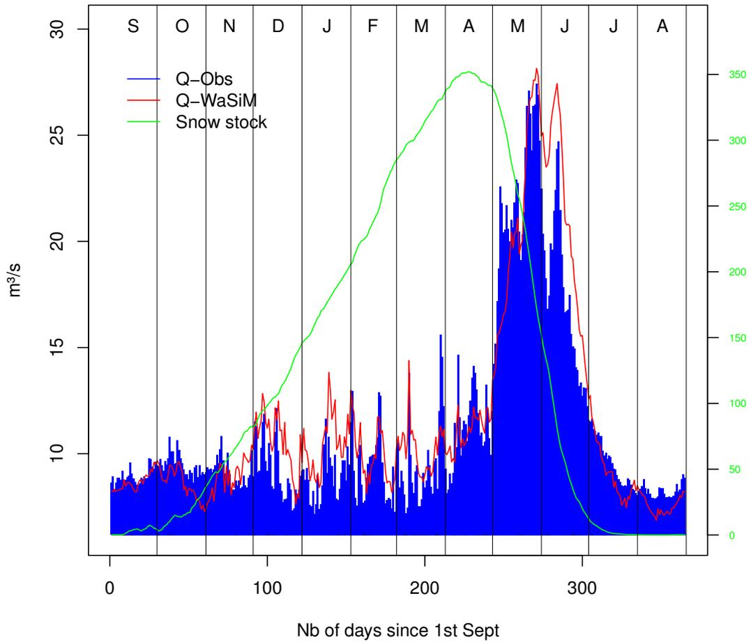
Figure 11. WaSiM-ETH model validation at gauge vhm10. Discharge seasonality: observed (blue), best model simulation (red). Simulated catchment-averaged snowpack (green) (mm SWE).
